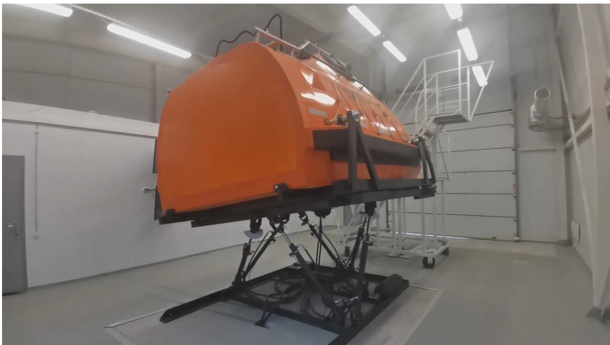
Dynamic platform provides lifeboat movement during free-fall launching and in rough sea
