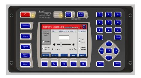
The imitator of DF-system RT-500M combines a communication direction finder and SAR (Search and Rescue) direction finder, thus allowing to bear all coastal and maritime radio stations. If equipped with an EPIRB (Emergency Position Indicating Radio Beacon), with its help person or vessels may be found quickly and safety.
