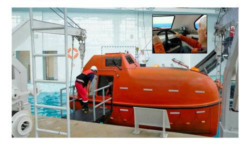
3D visualization system of the surfaced plant and specialized modified equipment (steering wheel, engine remote control handle, engine control panel) are implemented inside the cabin. These allow drilling the following practical skills:
