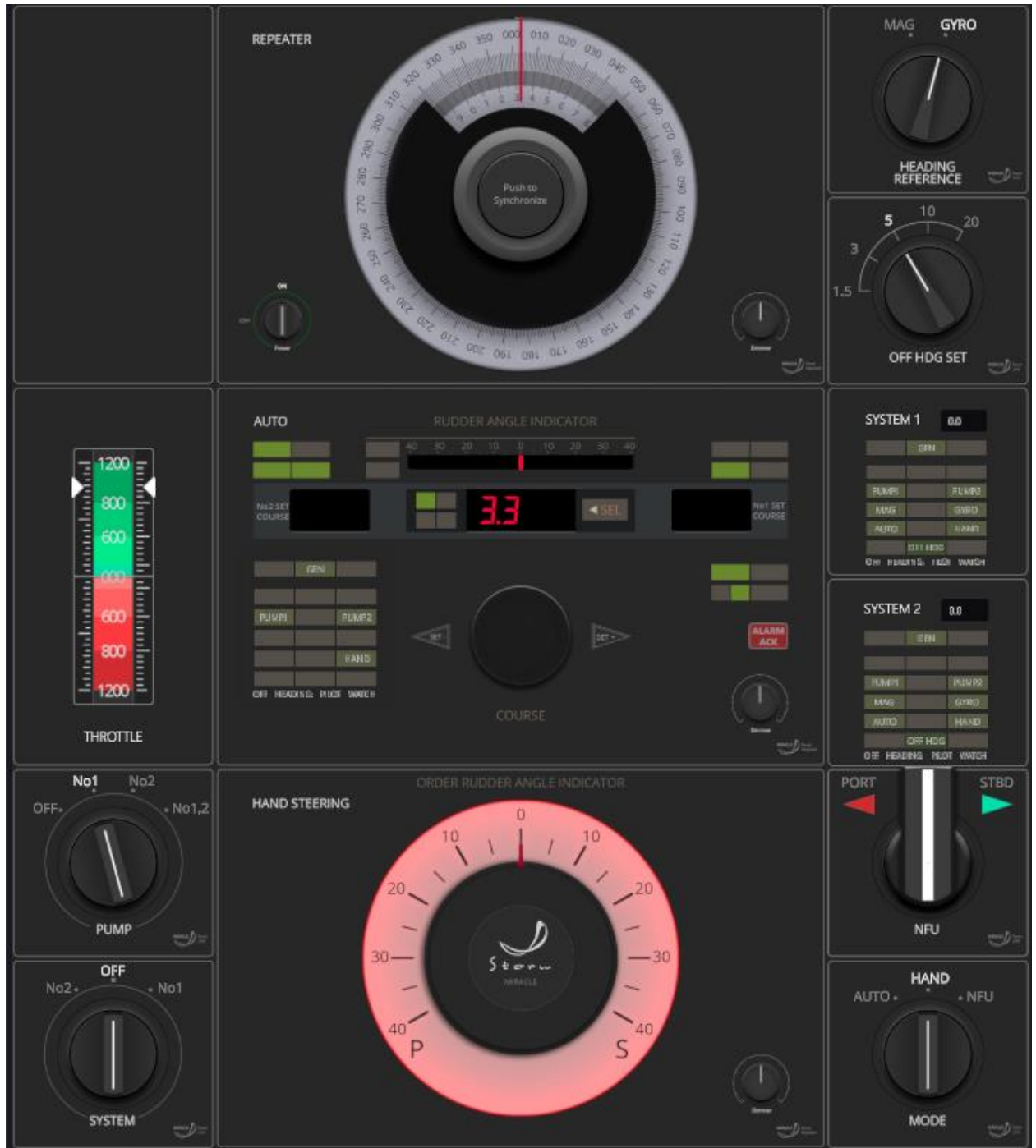
Autopilot system control panel
